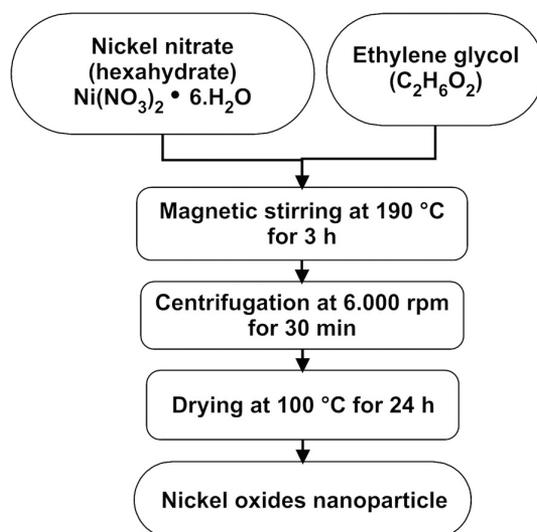
Figure 1. Flow diagram of the NiO nanoparticles preparation.
