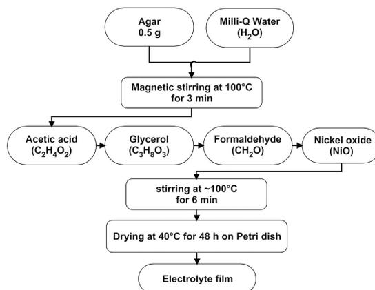
Figure 2. Flow diagram of the agar-NiO electrolyte preparation.
