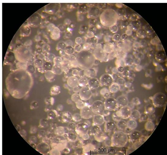
Figure 1. Optical micrograph of obtained PVAc microparticles.
