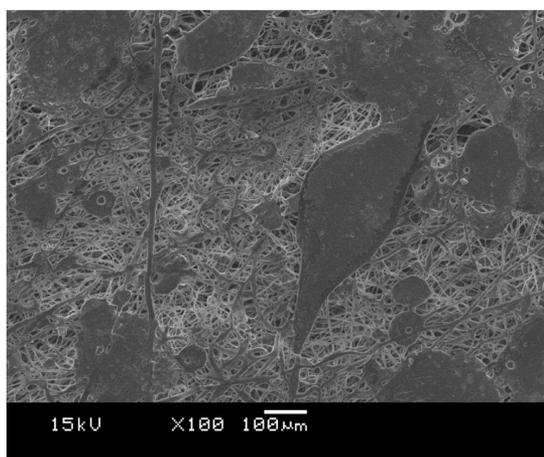
Figure 4. SEM of PCL500 sample.
