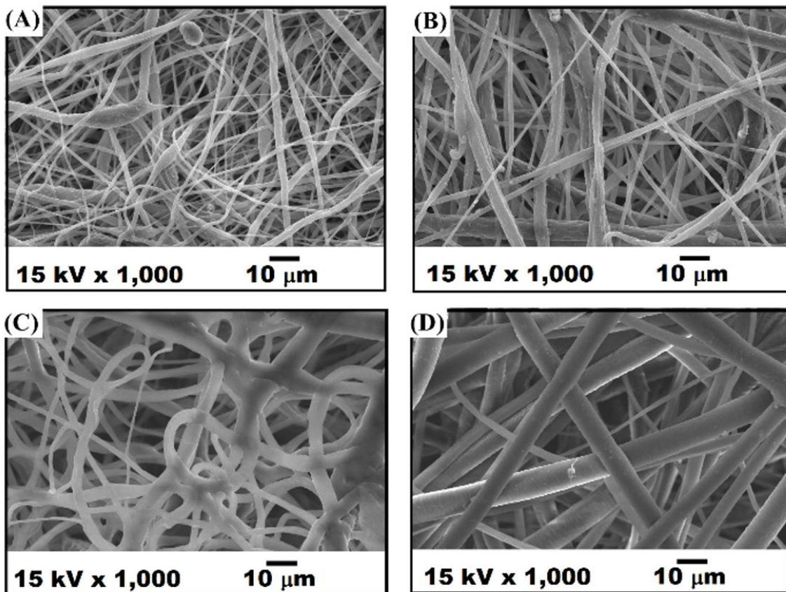
Figure 3. SEM of samples with different concentrations of oil and pure PCL, (A) 100 µg/mL, (B) 250 µg/mL, (C) 500 µg/mL and (D) PCL.
