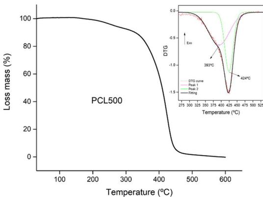
**Figure 6.** DTG curve for PCLT500 sample analyzed by least squares fit of gaussian functions.
