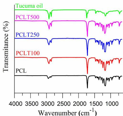
**Figure 2.** Infrared spectroscopy of PCL and PCL samples with 100  $\mu\text{g/mL}$ , 250  $\mu\text{g/mL}$  and 500  $\mu\text{g/mL}$  of tucuman oil.
