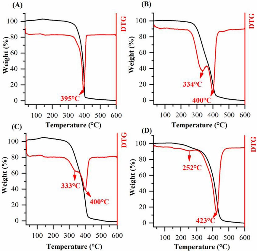
**Figure 5.** Thermogravimetric analysis (A) PCL, (B) PCLT100, (C) PCLT250 and (D) PCLT500.
