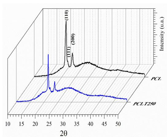
**Figure 1.** Diffractograms of pure PCL and PCL samples with 250  $\mu\text{g/mL}$  of tucuma oil.
