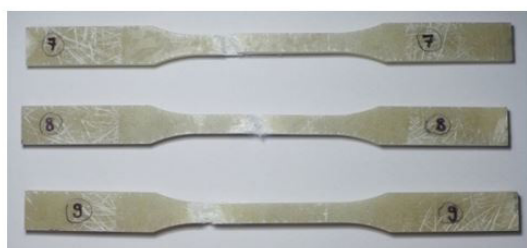
Figure 2. Image of sample scraps after rupture, in accordance with the numbering provided in Table 1 and Table 3.
