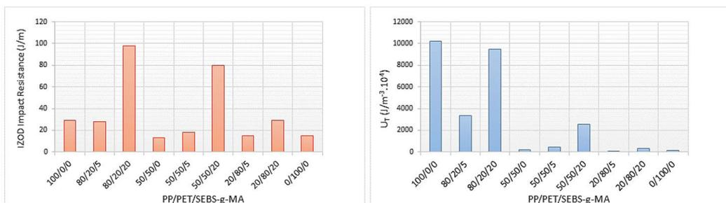
**Figure 9.** IZOD Impact Test results and Resilience Modulus ( $U_T$ ) and for all examined blends.
