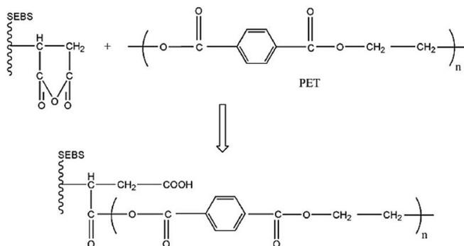
Figure 5. Interaction mechanism of maleic anhydride of SEBS-g-MA and PET<sup>[13]</sup>.
