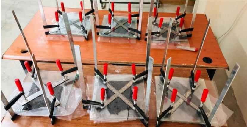
Figure 2. Hand lay-up method.
