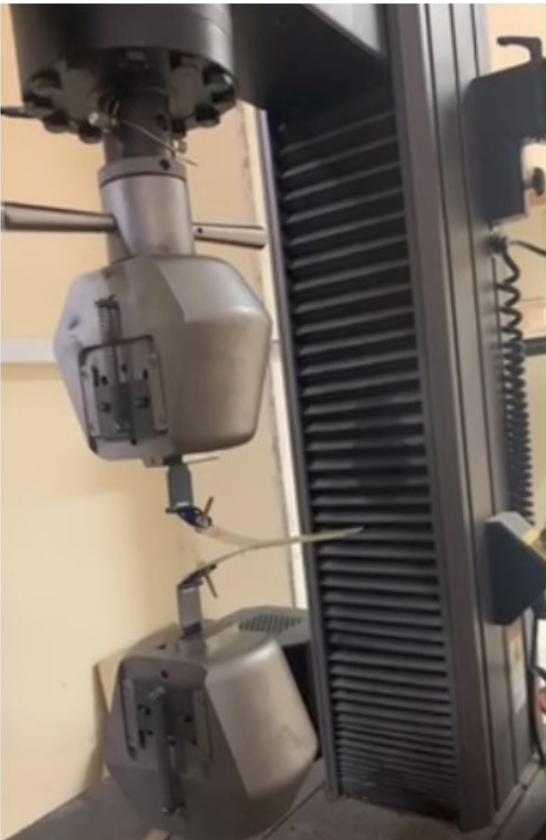
Figure 5. DCB test.
